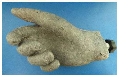
Figure 4 – Phantom hand used to assess the performance of the evaluation board (Figure 1) when regarding the human hand interaction.
