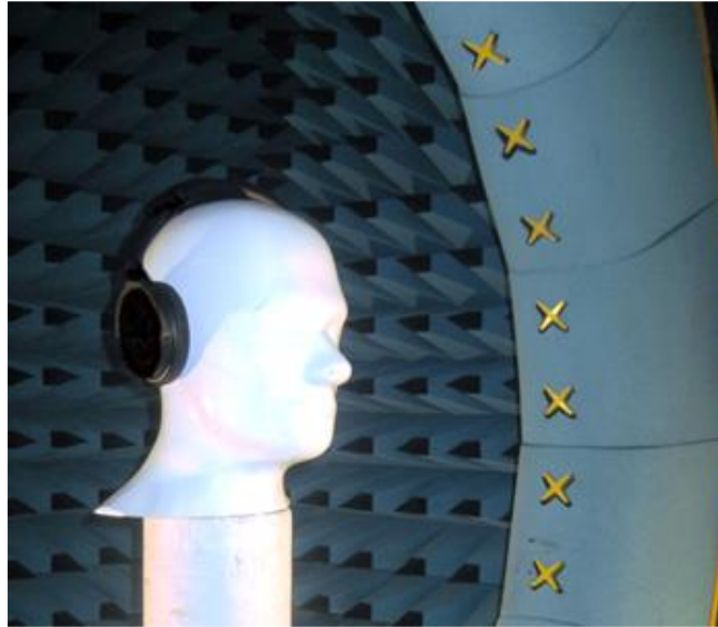
Figure 6. Antenna efficiency measurement of a headset in an anechoic chamber (3D pattern integration). Test includes a phantom head.
