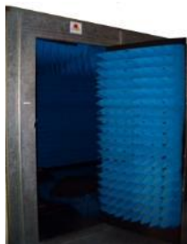
Figure 7. Anechoic chambers and full equipped in-house lab
