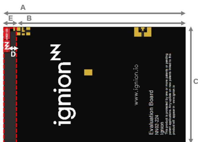
Figure 4 – EB_NN02-224-CR80-2400 in CR80 standard format. Evaluation Board providing operation from 2.4 GHz to 2.5 GHz.
