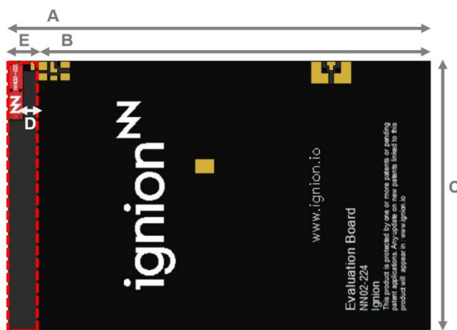
Figure 4 – EB_NN02-224-CR80-1561-1606 in CR80 standard format. Evaluation Board providing operation for BeiDou E1 band (1561 MHz), GPS L1 band (1575 MHz) and for GLONASS L1 band (from 1598 MHz to 1606 MHz).
