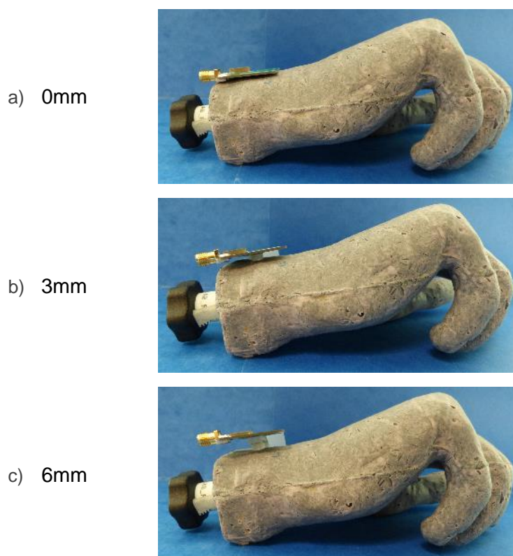
Figure 5 – Different distances between the phantom hand and the evaluation board that provide operation from 2.4GHz to 2.5GHz.
