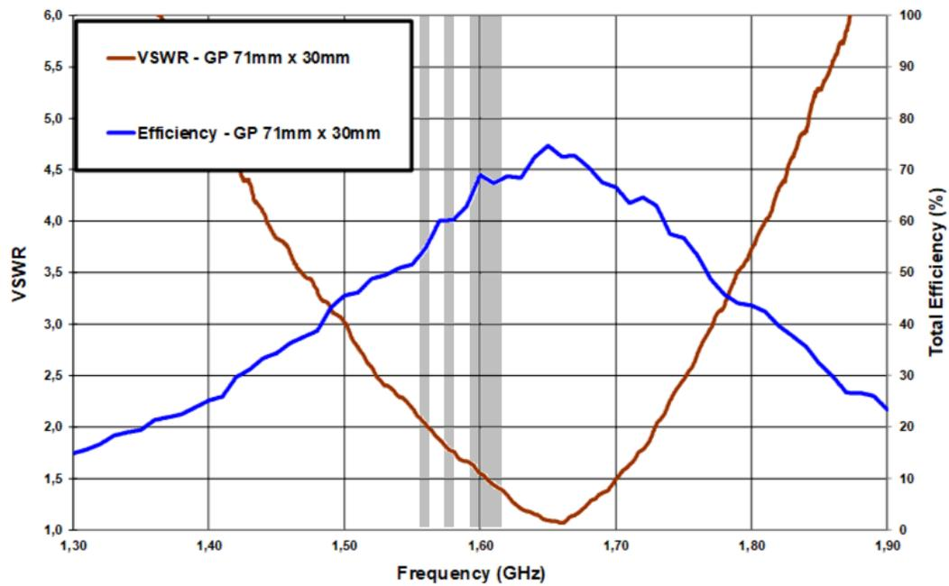
**Figure 3** – VSWR and Total Efficiency for BeiDou E1 band (1561 MHz), GPS L1 band (1575 MHz) and GLONASS L1 band (1598 – 1606 MHz) (from the Evaluation Board (Figure 1)).
