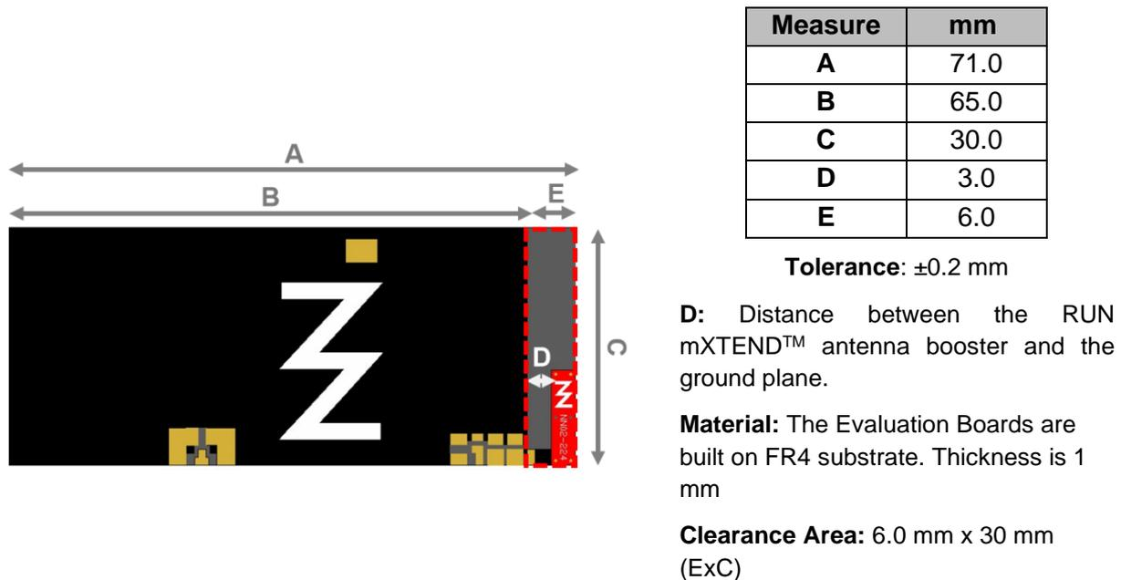
**Figure 1** – EB\_NN02-224-1561-1606 Evaluation Board for providing operation at BeiDou E1 band (1561 MHz), GPS L1 band (1575 MHz), Galileo E1 band (1575 MHz), and GLONASS L1 band (from 1598 MHz to 1606 MHz).
